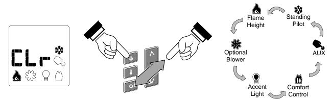
4 With the desired mode illuminated (the illustration below shows the AUX mode illuminated), press the "up" or "down" button to activate or clear the mode being addressed. Make sure to keep the on/off button depressed during this process.
