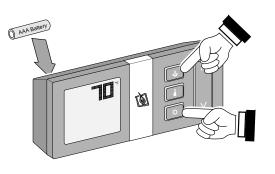
**<u>HINT:</u>** The easiest way to do this step is to place the top battery in the holder, slightly ajar. Then hold the the buttons down as you press the battery into place.
